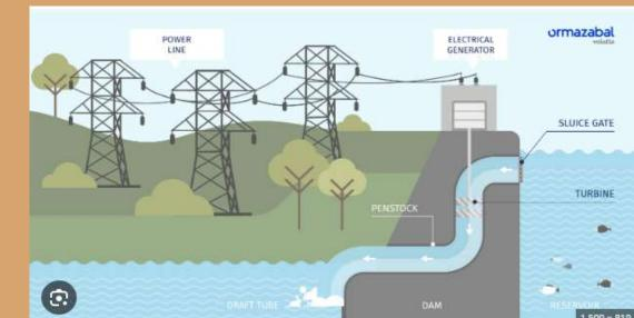
The falling water applies pressure against the turbine blades.
